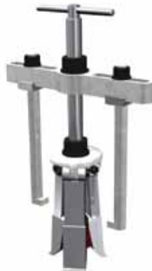
Fig 24: special wear ring pulling device Part no: 11004321
